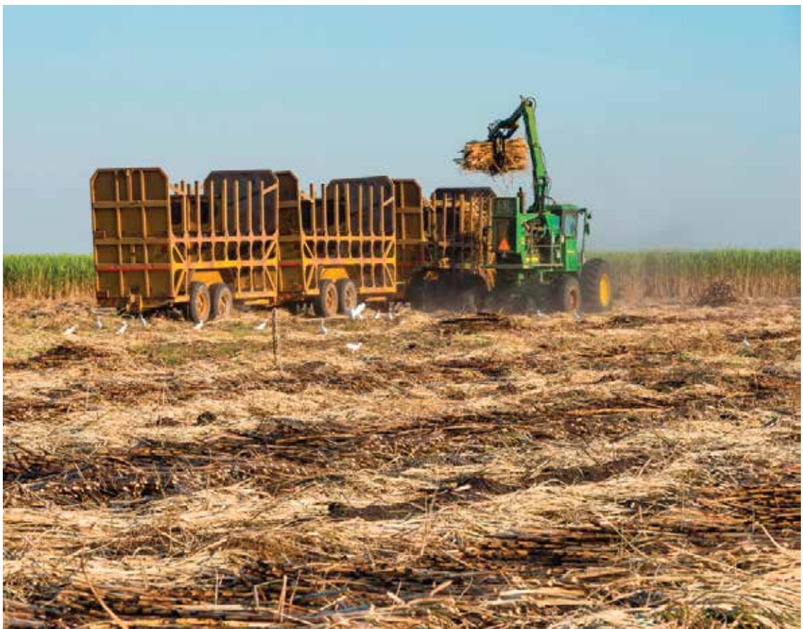
Infield loading with a grab loader
