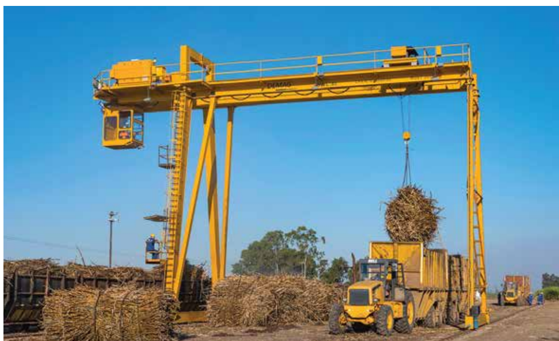
Overhead crane at a rail loading zone
