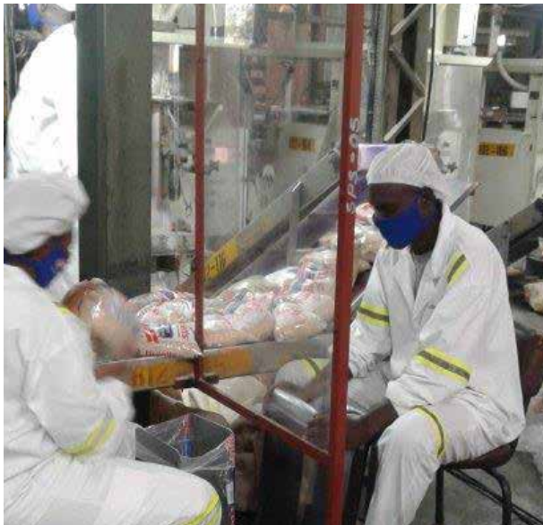
Screens installed to separate packers. The use of face masks is still being adhered with in addition to separation of work stations
