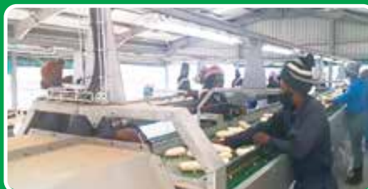
Seed cleaning involves the use of equipment to make various size and density separations of material so that the healthy seed is separated from the trash
