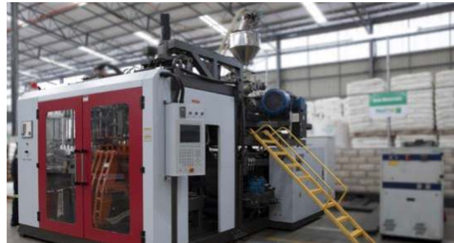
High Density Polyethylene (HDPE) bottle blowing machine
